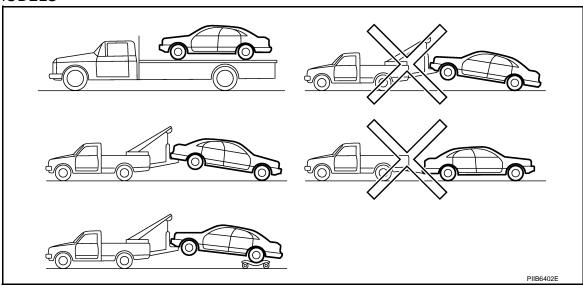
INFINITI recommends that vehicle be towed with the driving (rear) wheels off the ground or that a dolly be used as illustrated.
