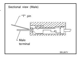
How to Check Enlarged Contact Spring of Terminal
